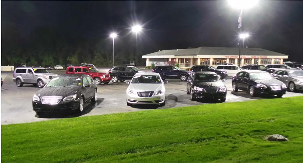
provide high levels of light but use substantially less energy. The front row poles originally used 2,674 watts based on two 1,000 watt and two 400 watt metal halides. We replaced them with one ARE-EHO LED that uses only 851 total watts a 78% reduction in energy usage.
